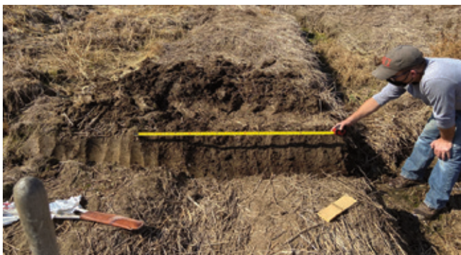
Researchers dissect the floodplain in a conservation ditch. Through the project, they established baseline geomorphology monitoring in conservation ditches to assess changes in shape through time.
